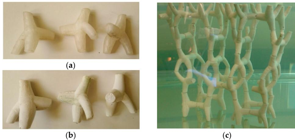
**Figure 10.** Prototyping the previously designed modules: (a) module prototype created using additive manufacturing and plastic; (b) module cast using concrete; (c) glued arrangement involving concrete parts, submerged in water.
